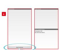
Bluetooth connection: Press Scan for devices to search. Find the device and enter default code:0000. Android Cell Phone Tunelinc Connect instruction
